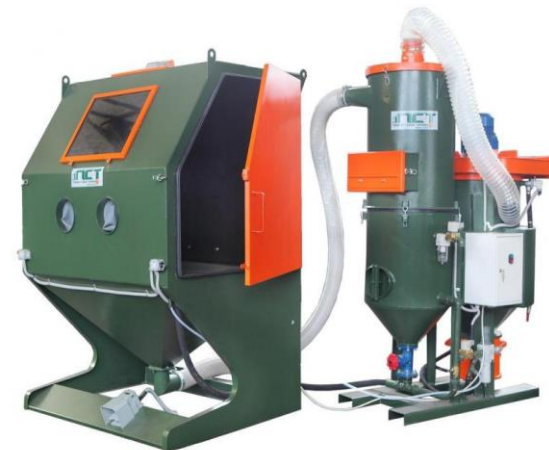
Installation for blowing the surface of a casting from ceramics and carbon deposits
