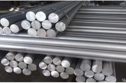
Initial rod of ZhS-6U-VI alloy (alloy grade “heat-resistant alloy improved by vacuum induction smelting”)
