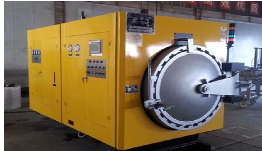
Boilerclave for removing model mass from the cavity of a ceramic mold
