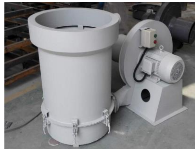
Sand powder with a pseudo-fluidized layer for applying a fire-resistant coating to a block of models
