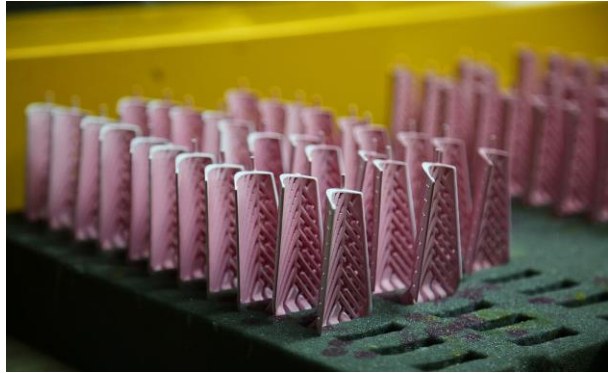
Ceramic rod for forming an internal cavity in a casting
